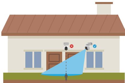
**i** Limited by PIR detection technology, the camera may fail to detect motion when environment temperature is close to human body temperature or someone approaches the PIR sensor vertically.
