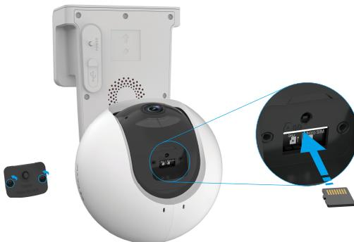
**i** After installing the Micro SD card, you should initialize the card in the EZVIZ app before using it.
